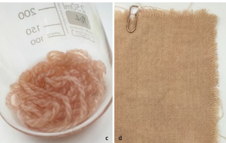
2 a Azaphilone colourants produced by Penicillium purpurogenum strains VTT D-99740 (liquid culture) or b VTT D-151592 (growth on agar plate) c were used for dyeing wool yarn and d fabric. Strain VTT D-151592 (= DSM 62866) was originally supplied by DSMZ GmbH. Yarn and fabric pictures by Monica Louise Gjøderum Hartvigsen
